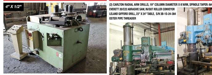
1998 IMCAR MODEL CPHV 100, B325279, 4" X 4" X 1/2" HYDRAULIC, HORIZONTAL & VERTICAL OPERATION, FLAT IRON UP TO 7", ROUND BAR 3", ADJUSTMENT OF LOWER ROLLS, VARI SPEED, SET OF ROLLS, S/N B325279
