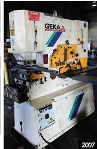
2007 GEKA HYDRACROP 110/A, HYDRAULIC, 120 TON, 12" PUNCH THROAT, 2" BAR SHEAR, 24" X 5/8" PLATE SHEAR, ASSORTED PUNCHES, S/N 21900
