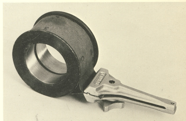
KKN-700 Universal Honing Fixture and HF-200 Workholder used to fixture Roller
